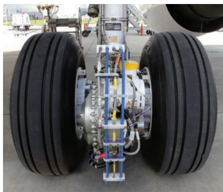
EGTS reduces aircraft fuel consumption and carbon emissions during ground operations.
